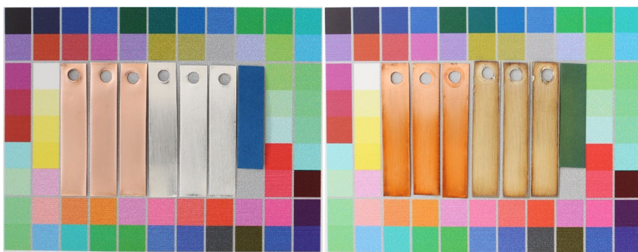
Fig. 5 Final design of colorimetric references with clean (left) and tarnished (right) copper and silver coupons
