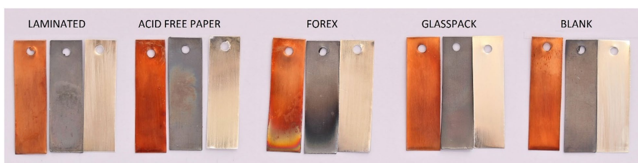
Fig. 4 Results from Oddy test on copper, lead and silver coupons exposed to laminated acid free paper, acid free paper, Forex Smart and Glasspack
